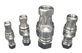
DOUBLE SHUT OFF QRC series is general purpose double shut off quick coupler capable of containing a wide variety of fluids. Puppet style having with captive puppet seal provides a Guaranteed leak free seal. Available in body size from 1/8 " to 3" with BSP, NPT thread standard.
